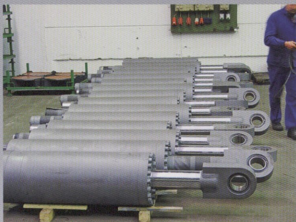
MAURER hydraulic dampers with 2,500 kN design force and 700 mm movement capacity for the Domovinski Bridge in Croatia
